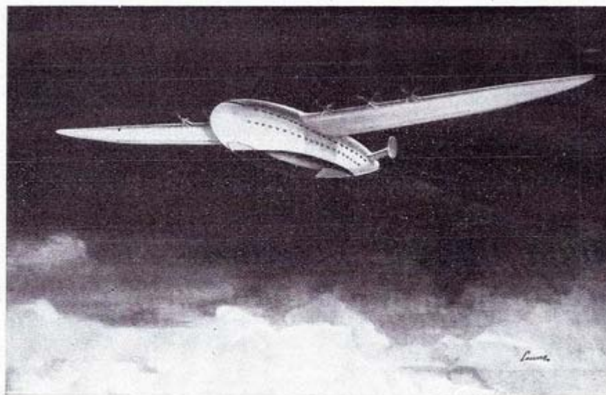
Artist's sketch of the proposed Sikorsky 100-passenger flying boat. This is one of a group of sketches included in the general design data recently submitted by Sikorsky Aircraft to Pan American Airways in connection with their request for bids for an airplane having a payload of 25,000 pounds capable of flying 5,000 statute miles at not less than 200 miles (322 km.) per hour.
